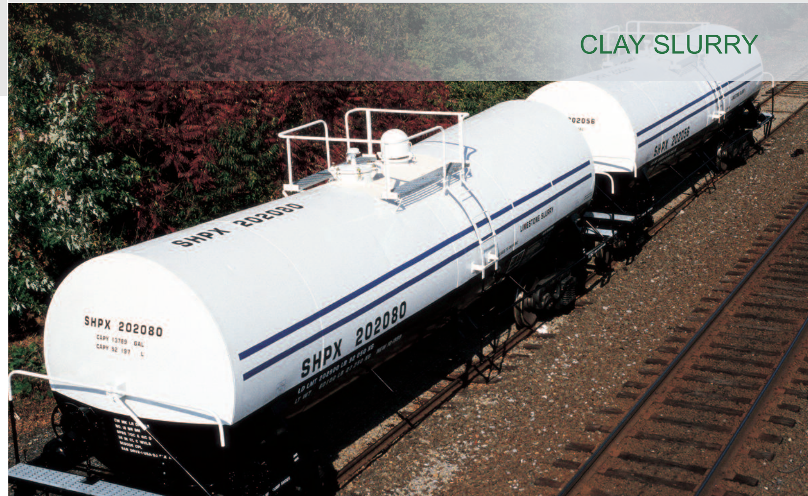
Tank car specifically designed for the transportation of clay slurry.
