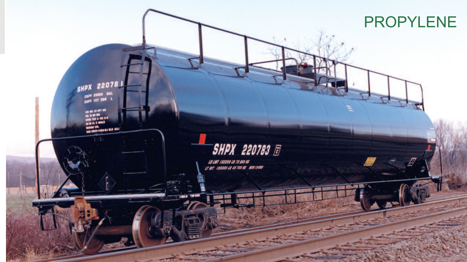
Tank car specifically designed for the transportation of propylene.
